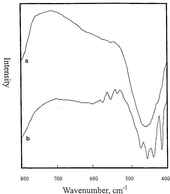
Figure 6. IR spectra of (a) MCM-41 and (b) MAS-5 after removal of organic templates.
